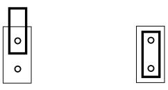
Jumper 2 in open position. Pre-wetting disabled. (Factory setting) Jumper 2 in closed position. Pre-wetting enabled.
